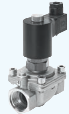
VZWF FORCE PILOT OPERATED SOLENOID VALVE 10 BAR MAXIMUM PRESSURE, 13.5 MM NOMINAL BORE
