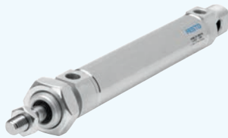
DSNU TO ISO 6432 DOUBLE ACTING WITH ELASTIC CUSHIONING RING 8 MM BORE
